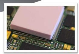
**UniGap 6000** is formulated with ceramic particles enabling extremely consistent and repeatable thermal performance. This in combination with stability over a wide range of operating temperatures makes **UniGap 6000** ideal for medical, aerospace and military applications.
