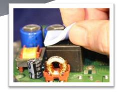
**UniGap 3000** is intrinsically tacky which excludes air at microscopic level and requires no additional adhesive. It has excellent compression performance over a wide range of stack up tolerances and applies minimal force to electronic components. **UniGap 3000** can be supplied with a fabric or film on one side for additional support during assembly.
