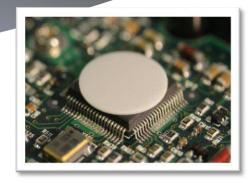
**UniGap 1000** is robust, highly flexible and easy to handle with 1.0 W/mK thermal conductivity. **UniGap 1000** has exceptional temperature stability and vibration dampening properties making it suitable for a wide range of rugged applications. **UniGap 1000** is used widely in automotive, LED, motor drive, PSUs applications plus many more.
